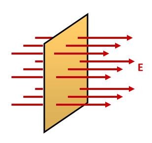
The **electric flux** passing through a surface is the number of electric field lines that pass through it.
