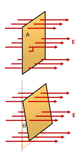
We define A to be a vector having a magnitude equal to the area of the surface, in a direction normal to the
