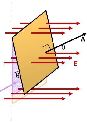
Because A is perpendicular to the surface, the amount of A parallel to the electric field is A  $\cos \theta$ .
